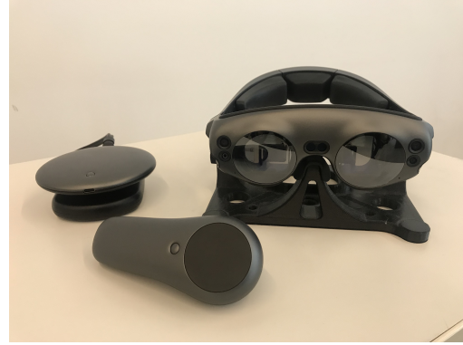
Figure 2. The OST AR headset being used in the system: Magic Leap One headset with a lightpack and a 6DoF controller
