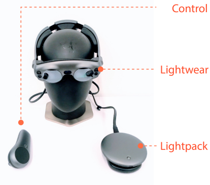
Figure 1. The Magic Leap One, an Optical See-Through, Head-Mounted Display (OST-HMD). We use the eye tracking and head pose tracking the lightwear provides and the 6DOF control to create visual annotations. To add more context information into asynchronous communication, we record spatial audio.
