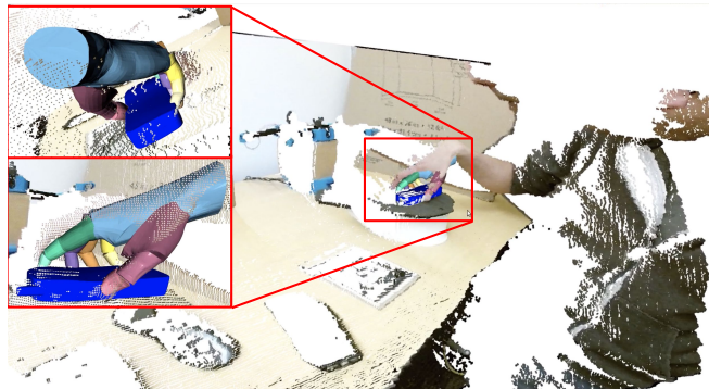
Figure 1: Grasp capture for a scene depicting a cellphone being grasped. The multi-colored hand model shows the estimated hand pose and the dark blue model shows the estimated object pose.
