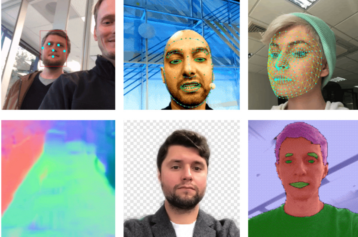
Figure 3. Real-time AR effects using TFLite GPU (best viewed in color). Upper row: (a) Left: Fast Face Detection; 200Hz on Pixel 1. (b) Center: 2D Contour; 50Hz on Pixel 2. (c) Right: 3D Face Mesh; 280Hz on iPhone 7. Lower row: (d) Left: Normal Map Prediction; 10Hz on Pixel 2. (e) Center: Background Segmentation; 40Hz on Pixel 2. (f) Right: Multi Segmentation; 40Hz on Pixel 2.
