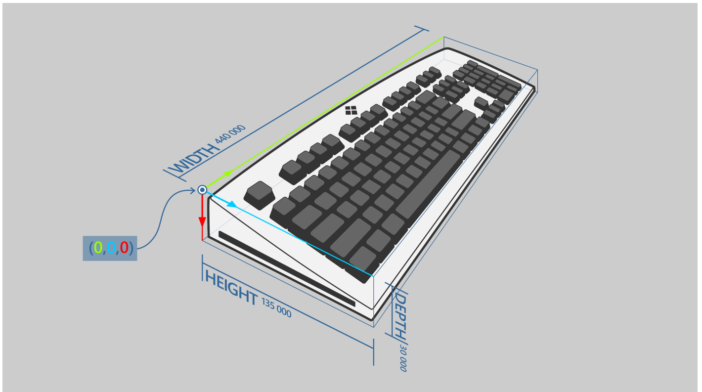
Figure 24.2: Keyboard with labeled dimensions and origin. Lamps exist beneath every key, the branding at the top/middle, and accent lighting along the left and right sides. Example sizes given for each dimension (in \mu\text{m} ).
