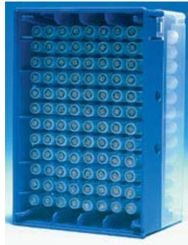
Figure 2.4.1a: 2D bar-code labelled 1.4ml aliquot storage tube (without seal); and Figure 2.4.1b: 96 x 1.4ml tubes in SBS footprint storage rack 2.4.2.2 EDTA Plasma Separator Tube (PST) vacutainers
