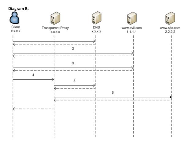
**Diagram B** visualizes an attack flow when a transparent proxy using Approach B is located between a client and an evil website. The preface for this would be a user visiting a malicious website, or a website with malicious ad which spawns an iframe to an attacker controlled destination.
