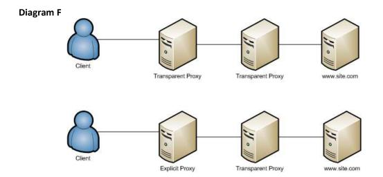
Diagram F outlines chain configurations which are not vulnerable to 'Approach A'.
