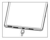
You are advised to fully charge the battery (**(**). Charging status is indicated by a percentage displayed on the screen. The percentage increases as the device is charged.
