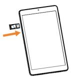
**Step 4.** Slide the tray slowly into the SIM tray slot. It only fits one direction. Do not force into place. Keep the SIM tool in a safe place for future use.
