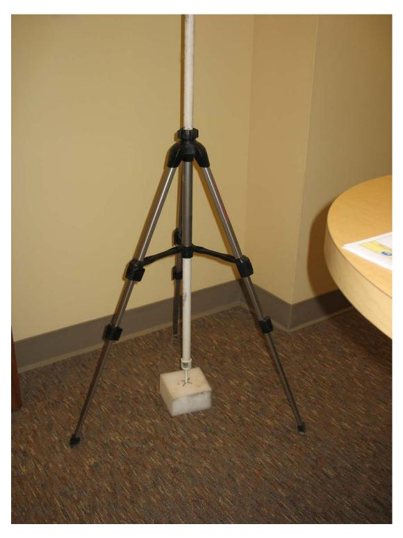
The photographic tripod (SLIK model #U2000) has the original center camera-mount barrel removed. The center hole of the tripod  $\underline{\text{must}}$  then be drilled out to 7/8-inch  $\underline{\text{diameter}}$  to allow the  $\frac{1}{2}$ -inch PVC pipe to be inserted.
