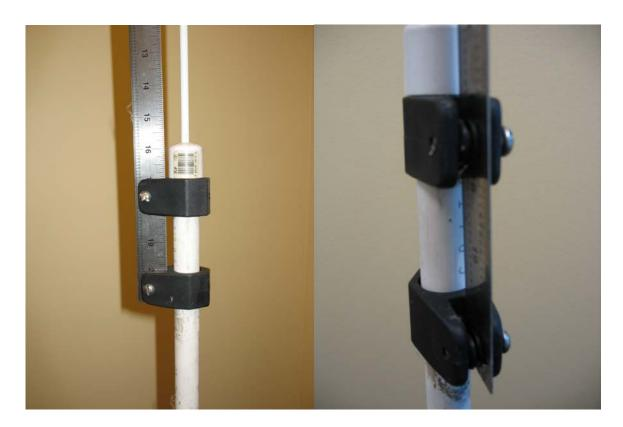
The top slip cap (and bottom slip cap) on the PVC barrel are center drilled with a 5/16-inch hole for the sliding fiberglass rod (1/4-inch diameter by at least 60 inches long). The 24-inch stainless steel ruler is fixed to the top of the PVC barrel using 7/8-inch Bimini Rail Mounts (and ¼-inch-diameter rubber hole grommets as spacers, seen in photo on right). Drill the ruler to fit the Rail Mounts.
