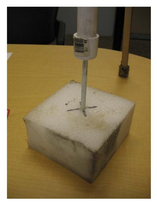
The bottom slip cap (and top slip cap) on the PVC barrel are center drilled with a 5/16-inch hole for the sliding fiberglass rod (1/4-inch diameter by at least 60 inches long). The foam block consists of closed-cell foam, cut to approximately 4-inches square by 2-inches thick (your block size may vary), with a center drilled 3/16-inch hole (only through the top half of the block) for the fiberglass rod.
