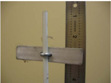
The flat aluminum bars are attached to the top of the fiberglass rod with the wire rope clip, one aluminum bar on each side of ruler. Several washers are on arms of wire rope clip, separating the two aluminum bars to allow them to slide freely along ruler as water level falls.
