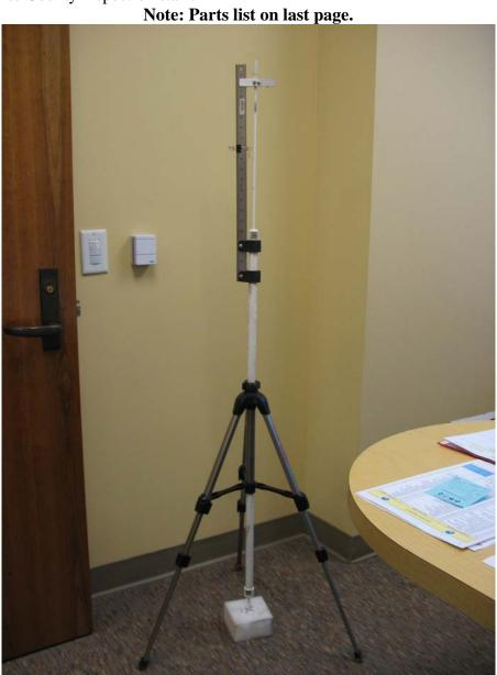
The percolation test measuring device consists of a modified photography tripod with a PVC barrel guiding a sliding fiberglass rod. A stainless steel ruler is attached to the top of the PVC barrel to measure the changing water level in the percolation test hole. The sliding rod has a closed cell foam block on the bottom as a float, and aluminum plates attached to the top of the fiberglass rod to aid in measuring water level changes.
