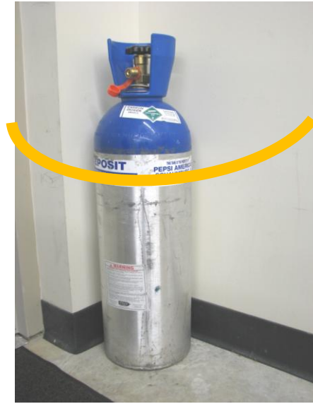
Even small compressed gas cylinder can become lethal rockets when the valve is knocked off!
