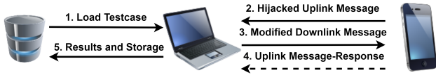
Figure 4: Testing Flow. Our testing approach focuses on modifying downlink messages towards the UE (Step 3).
