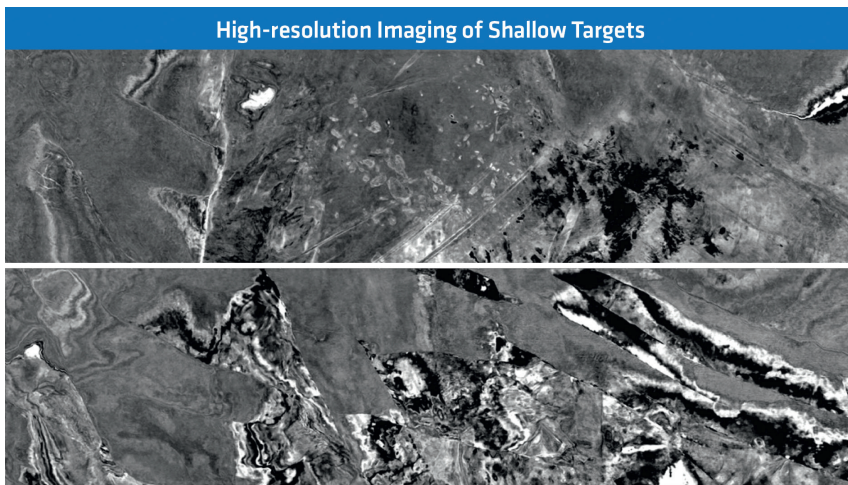
Figure 5 High resolution imaging results of the near-surface do not show any acquisition footprints typically caused by near-offset gaps at sail line boundaries. The depth slices shown are extracted from 410 m and 468 m below main sea level. Water depth ranges from 300 m to 400 m in the area. The surface dimensions of the depth slices are 21.9 km x 5.3 km. The ultra-wide penta source set up provided a natural processing bin size of 6.25m x 6.25m and uniform sampling of the ultra-near offsets.
