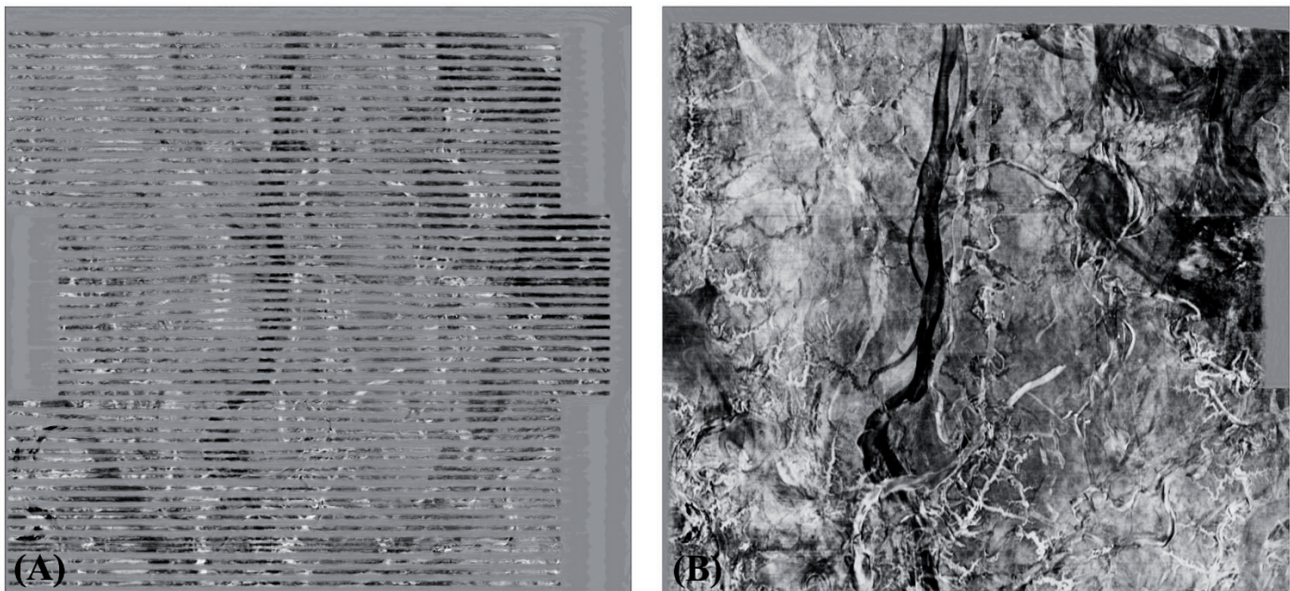
Figure 8 Depth slices at 105 m below sea surface from imaging of primaries (A) and imaging of multiples (B). The image from multiples not only includes greater coverage of the subsurface at this depth but the image also includes details that are not present in the primary wavefield image. Imaging of multiples enhances subsurface imaging illumination and resolution.
