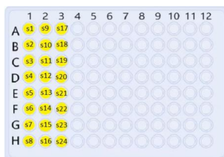
Figure 1. 24 sample input plate example for SRE (s1–s24). Prepare in the 96-well PCR 200 \mu L plate (Bio-rad, HSP9601).
