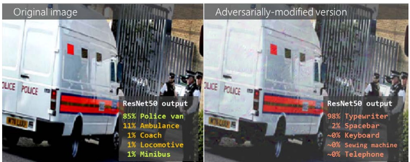
Figure 21 – An image classifier can be subverted by making changes which are almost imperceptible to the human eye (SOURCE: Cambridge Consultants)
