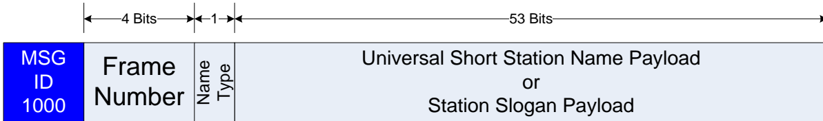
Figure 4-24: General Message Structure for MSG ID 1000
