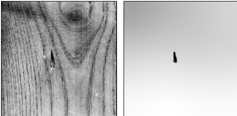
Figure 5.8: Defect detection in wood. (a) LEFT: Wood surface, \Omega = (0, 256)^2 . (b) RIGHT: Isotropic nonlinear diffusion, \lambda = 4 , \sigma = 2 , t = 2000 .
