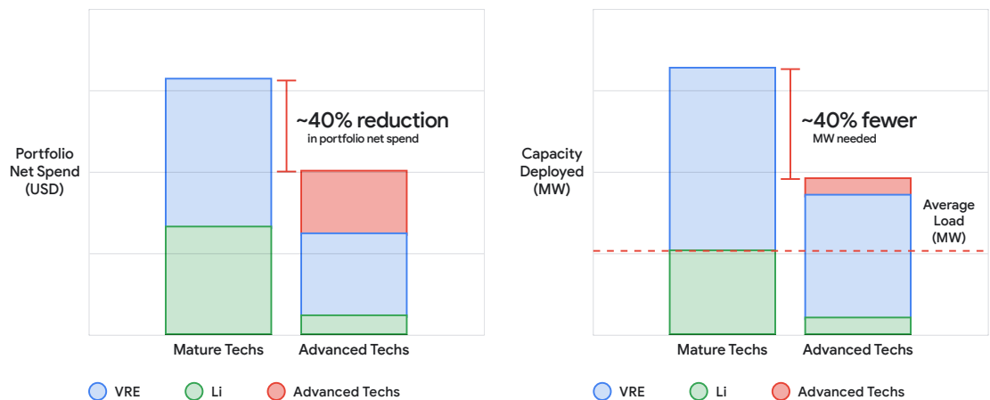
FIGURE 3: Cost (left) and capacity (right) comparison between Mature Technologies and Advanced Technologies scenarios in Google’s CFE Optimization Model for 90% CFE across global portfolio.
