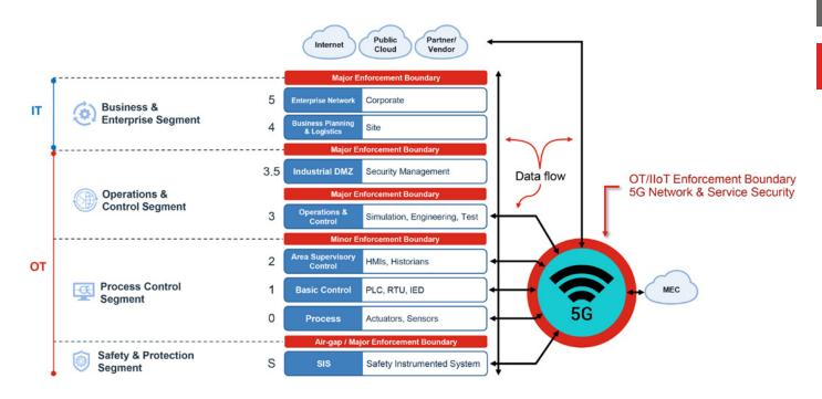
Figure 2: Enhancement to ISA99 Purdue reference architecture in a 5G industrial environment.
