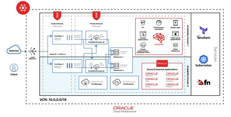
Figure 2: Reference architecture for securing Oracle applications with Fortinet solutions on OCI.
