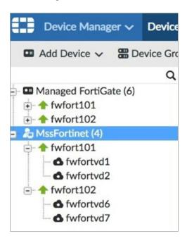
Here, 'MssFortinet' is the device group, which has the following VDOMs as members:
