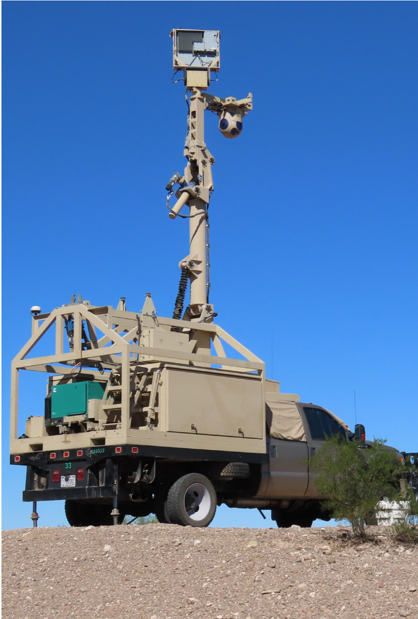
A Mobile Surveillance Capability (MSC) vehicle in Pima County, Arizona. This model made by FLIR is sometimes referred to as a Mobile Video Surveillance System (MVSS). Source: EFF.
