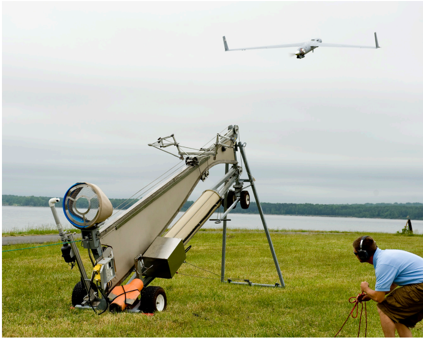
Insitu Scaneagle with launcher. Source: U.S. Coast Guard.
