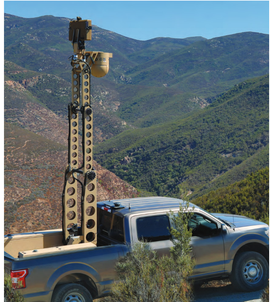
A Teledyne FLIR Lightweight Vehicle Surveillance System (LVSS), also known as a Mobile Surveillance Capability Lite (MSC-Lite). Source: USBP.
