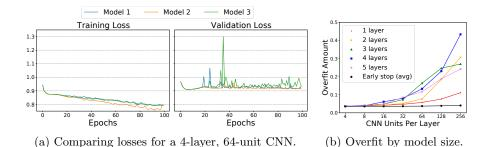
Fig. 6. On left (a): the training and validation loss for a 4-layer, 64-unit CNN, across random seeds. On right (b): the average overfit amount without early stopping, shown for all CNN sizes, compared to the average overfit amount for all layers with early stopping.
