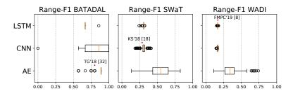
Fig. 5. The final range-F1 scores of each model when trained and tuned on 3 experimental ICS datasets. For each dataset, a selected model hyperparameter setting from prior work is included for comparison.
