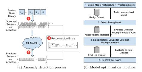
Fig. 2. The anomaly-detection process is shown on the left: a sequence of system states is reconstructed by an ML model, and high reconstruction errors are used to identify anomalies. The optimization pipeline for the anomaly-detection process is shown on the right, with each optimization step and its relevant datasets.
