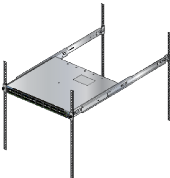
Figure 15: Attaching the Switch to the Rack Posts
