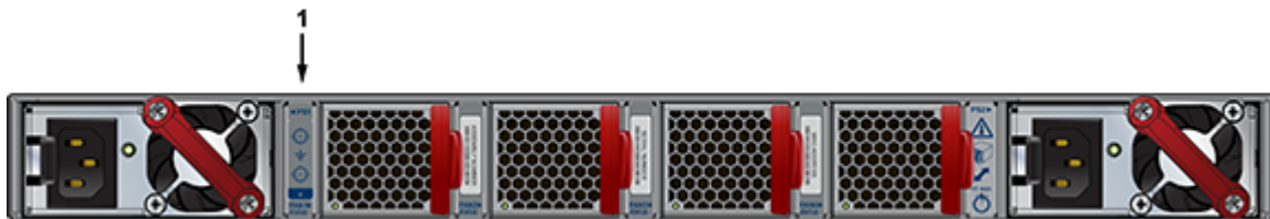
Figure 16: Earth Grounding Pad Sockets for Models without Management Ports on the Rear Panel
