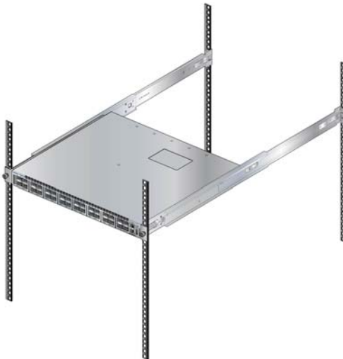
Figure 3-12: Attaching the Switch to the Rack Posts
