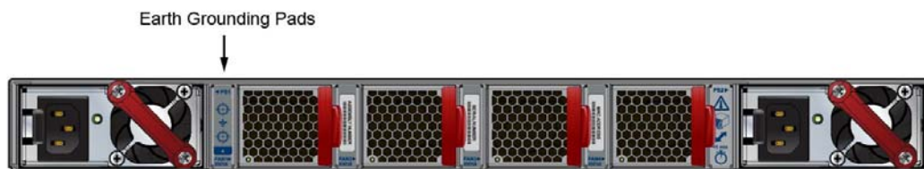
Figure 4-1: Earth Grounding Pad Sockets for Models without Management Ports on the Rear Panel
