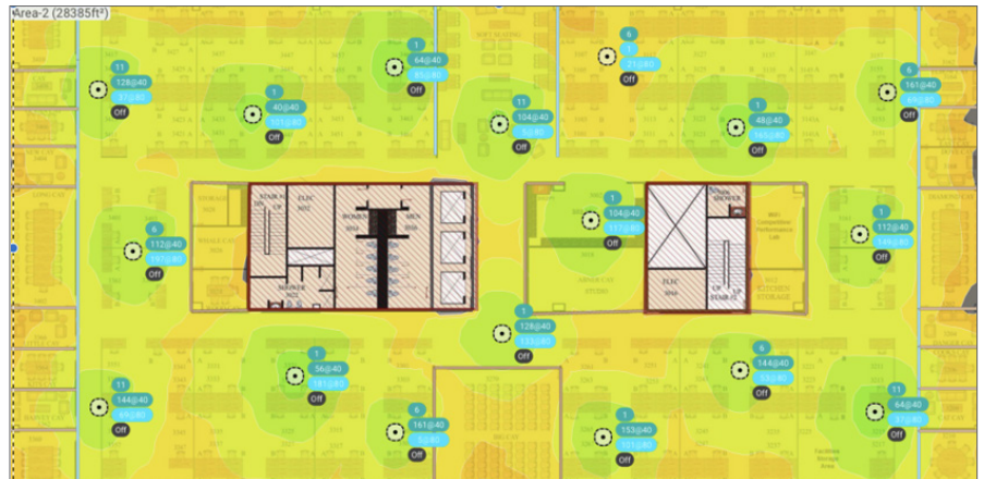
Figure 1: Floor plan of HQ location wherein 17 APs were replaced with C360 11ax
