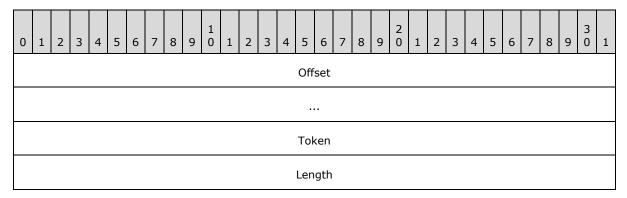
**Offset (8 bytes):** The RDMA provider-specific offset, in bytes, identifying the first byte of data to be transferred to or from the registered buffer.
