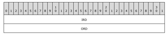
**IRD (4 bytes)**: The Incoming RDMA Read Depth currently in use by the sending peer on the connection. This value MUST be greater than zero.
