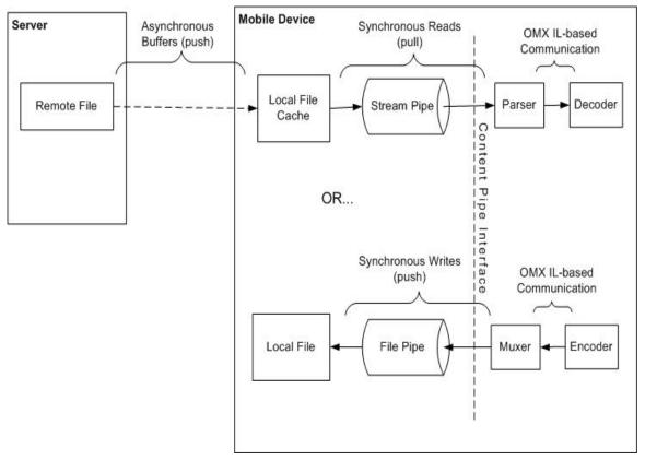
Figure 1: Content Pipe Operation Example - OpenMAX IL
