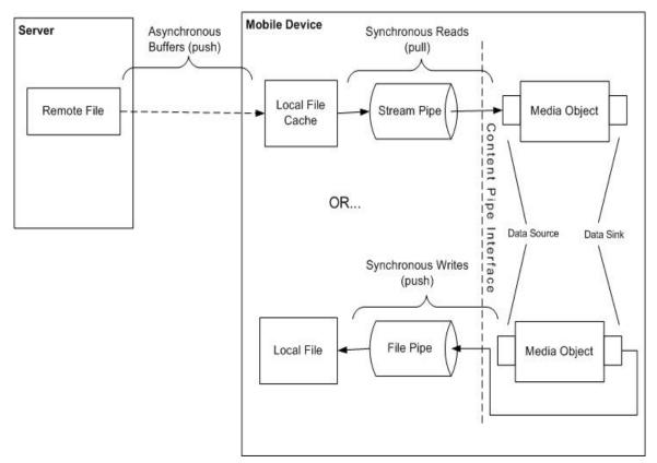
Figure 2: Content Pipe Operation Example - OpenMAX AL/OpenSL ES
