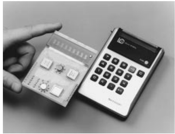
Fig. 13. The first liquid-crystal pocket calculator, which used DSM. Courtesy of Sharp Corporation.
