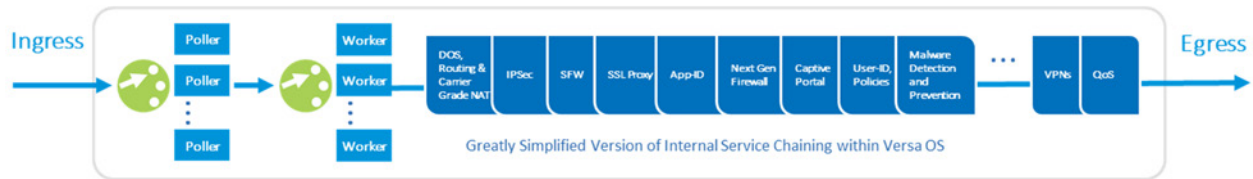
Figure 6. Versa Single Pass Architecture.
