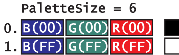
Figure 129. Palette Structure of a Black & White, One-Bit Image
