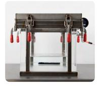
To test for IPX7/8 water immersion protection, Apple submerges iPhone inside a pressurized vessel to simulate pressure experienced underwater.
