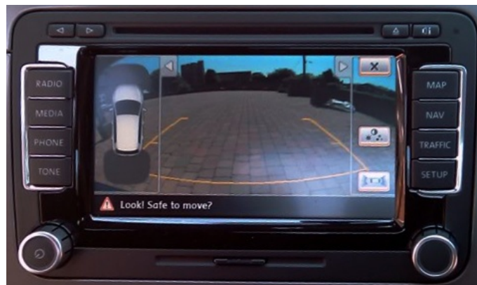
Figure 1.1: Optical parking system for a car
