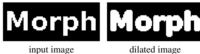
Figure 5.3: Binary dilation according to Listing 5.2
