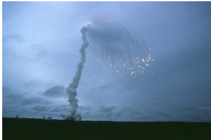
Figure 1.7: Ariane 5 disaster caused by numerical overflow
