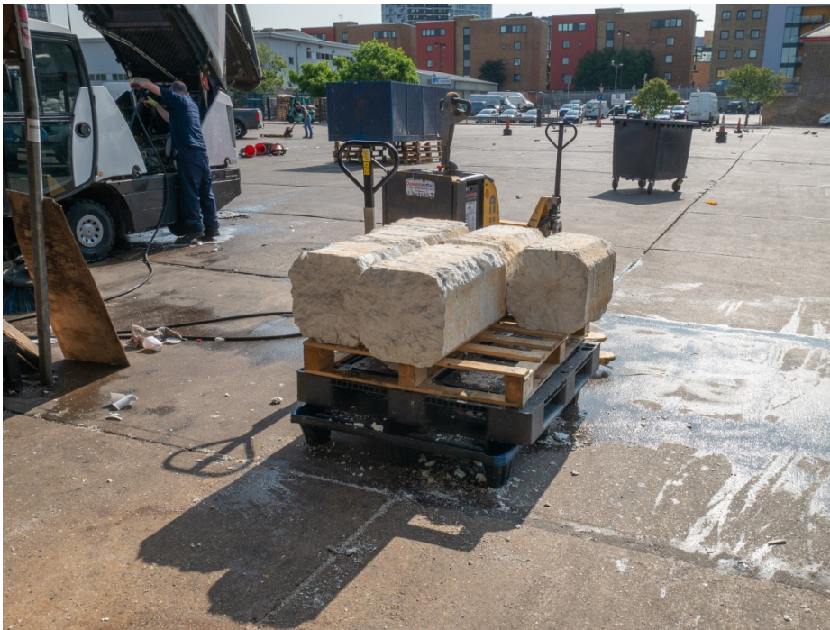
Figure 297. Photo - Briquettes of compressed EPS being added to a pallet
