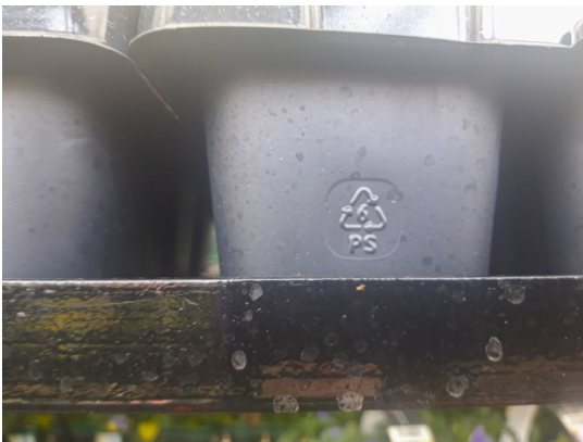
Figure 21. Photo - Black PS plant trays in use in Ireland (Credit: Maeve Thornberry)
