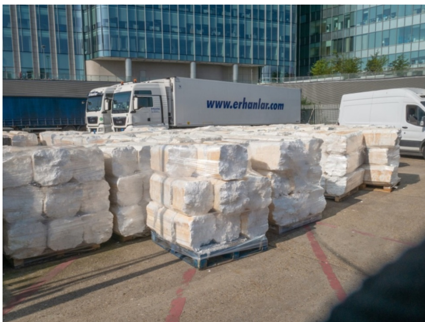
Figure 28. Photo - Pallets of compacted EPS briquettes at Billingsgate Market (Credit: Maeve Thornberry)
