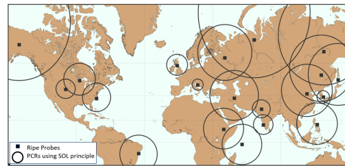
Fig. 4. Detecting IP anycasting. Dots represent the RIPE probes and circles represent the distance estimated to the IP address based on speed of light constraint.
