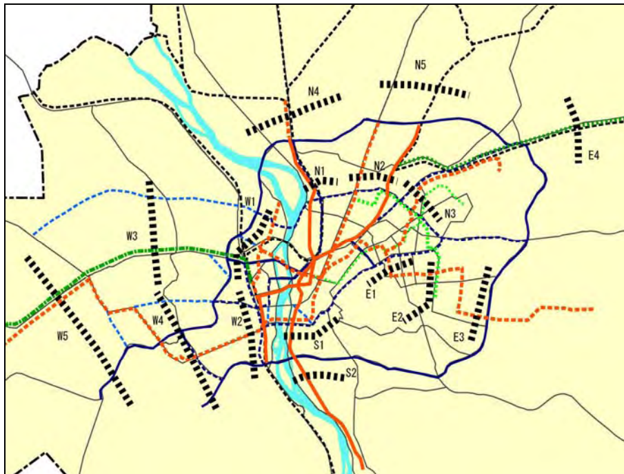
Figure 4.5.2 Cross Sections Applied for Demand/Capacity Assessment
