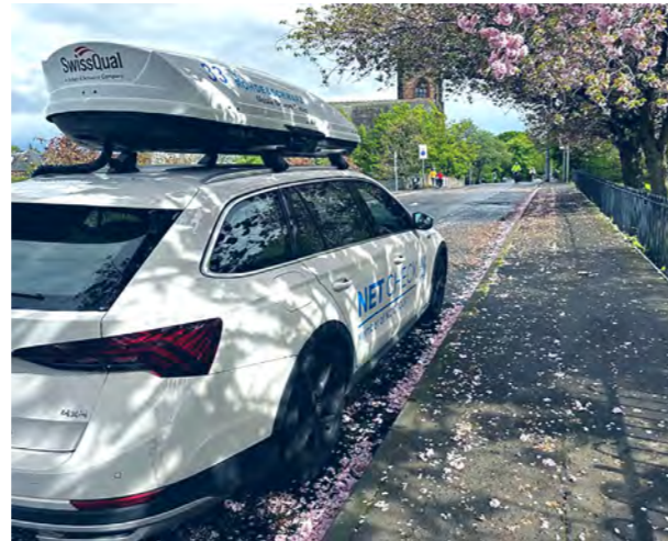
NET CHECK drive testing
