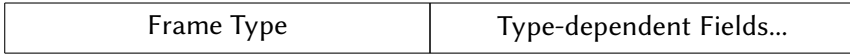
Figure 4.3: Format of a QUIC frame. The Frame Type field is a variable-length integer.
