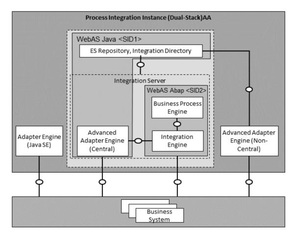
Figure 4: System Landscape for Building Integration Scenarios with PI Standard Installation
