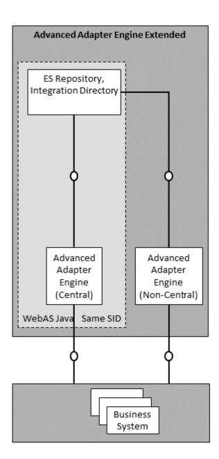
Figure 5: System Landscape for Building Integration Scenarios with Advanced Adapter Engine Extended (AEX)
