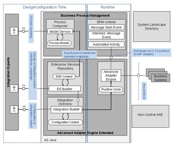
Figure 6: Components of Process Orchestration
