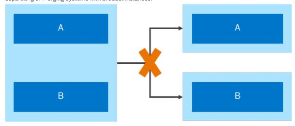
Figure 13: Separating systems with product instances are not supported with SAP standard system copy and migration tools
