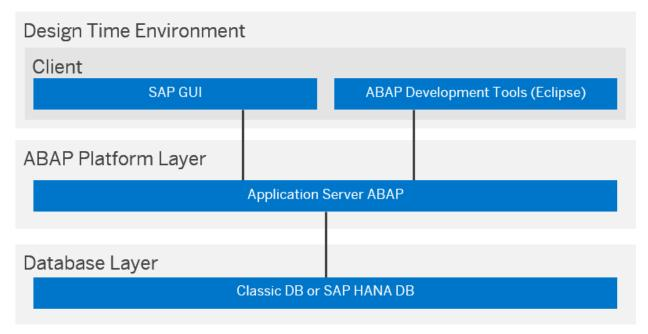
Figure 11: Software layers and components that are used in the Custom Application Development scenario
