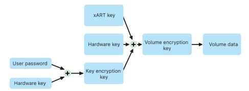
On a Mac with Apple silicon and those with the T2 chip, all FileVault key handling occurs in the Secure Enclave; encryption keys are never directly exposed to the Intel CPU. All APFS volumes are created with a volume encryption key by default. Volume and metadata contents are encrypted with this volume encryption key, which is wrapped with the class key. The class key is protected by a combination of the user's password and the hardware UID when FileVault is turned on.
