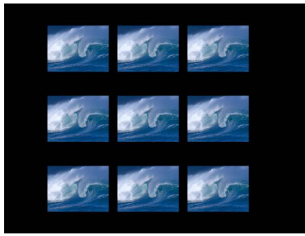
Rectangle replicator shape with Origin set to Top and Source Frame Offset set to 0
