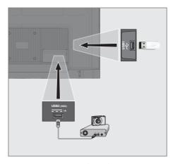
1 Connect the USB2 (HDD) interface of the television and the corresponding socket on the data device (external hard drive, digital camera, card reader or MP3 player) using a USB cable;
