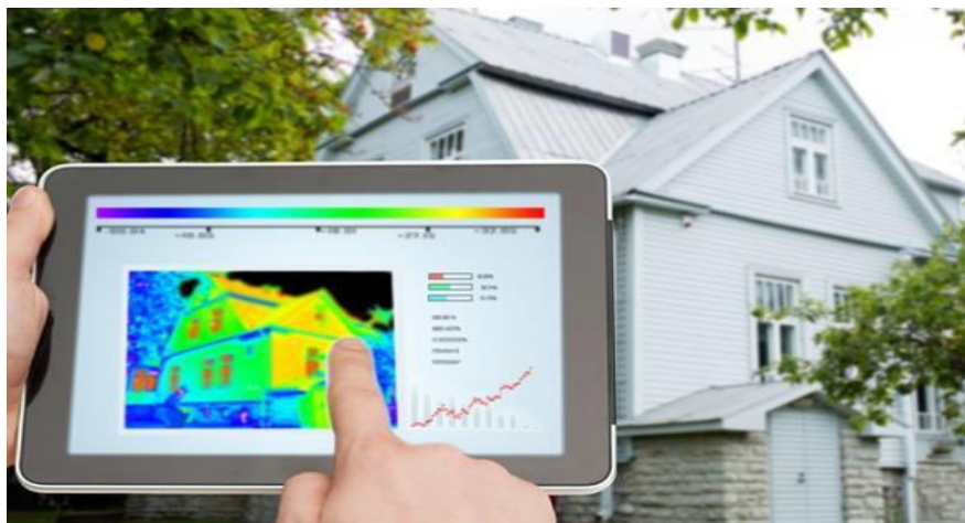
Figure 2: A thermographic representation of a building to detect air leaks and insulation gaps
