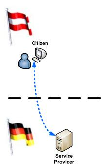
In the middleware model the Service Provider uses software components (a middleware "SPware") that implement a direct communication with the foreign eID token.
