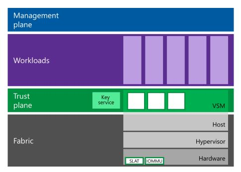
Figure 1 – visual diagram of the 'trust plane' concept
