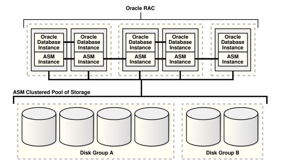
A clustered storage pool can be shared by multiple single-instance Oracle Databases as shown in Figure 1-3. In this case, multiple databases share common disk groups. A
