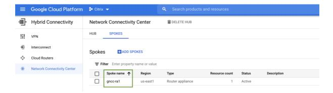
Alternatively, the Spoke can be attached to the Hub in the UI by going to "Hybrid Connectivity > Network Connectivity Center > Spoke" section as shown in the screenshot above.
