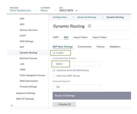
Configure two BGP Peers pointing to two separate interfaces (10.0.4.10 and 10.0.4.11) of the Cloud Router as show below.
