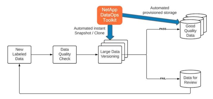
The NetApp DataOps Toolkit complements the data quality-checking pipeline through the use of its near-instantaneous data cloning technology. Each labeled file must be assessed and compared to the existing labeled files. Distributing these quality checks across various data storage systems ensures that these checks are executed quickly and efficiently.
