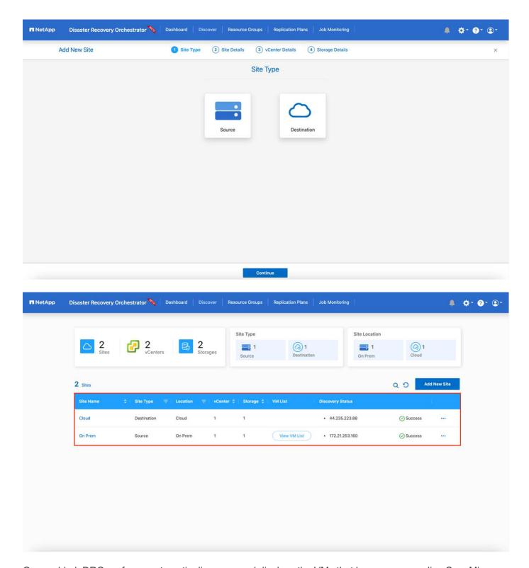
Once added, DRO performs automatic discovery and displays the VMs that have corresponding SnapMirror replicas from the source storage to FSx for ONTAP. DRO automatically detects the networks and portgroups used by the VMs and populates them.
