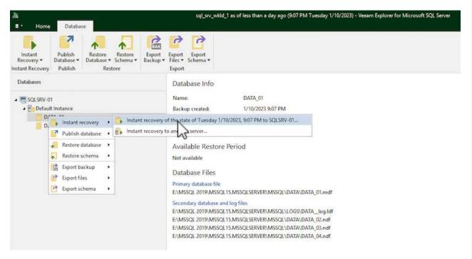
5. In the Instant Recovery Wizard specify the switchover type. This can either be automatically with minimal downtime, manually, or at a specified time. Then click the **Recover** button to begin the restore process.
