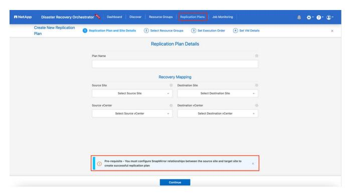
3. After Recovery mapping is completed, select the cluster mapping.
