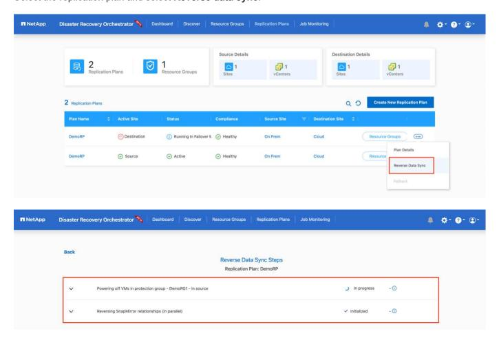
Once completed, you can trigger failback to move back to original production site.
